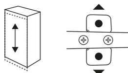
Adjust the height of the front by loosening these screws and pressing the mounting plate up or down.
