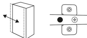
The outer screw on the hinge arm adjusts the front sideways. You can also level the front by simply adjusting this screw on one of the hinges.
