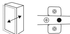
The inner screw of the hinge arm adjusts the depth of the front, i.e. how far out from the frame the front should sit.
