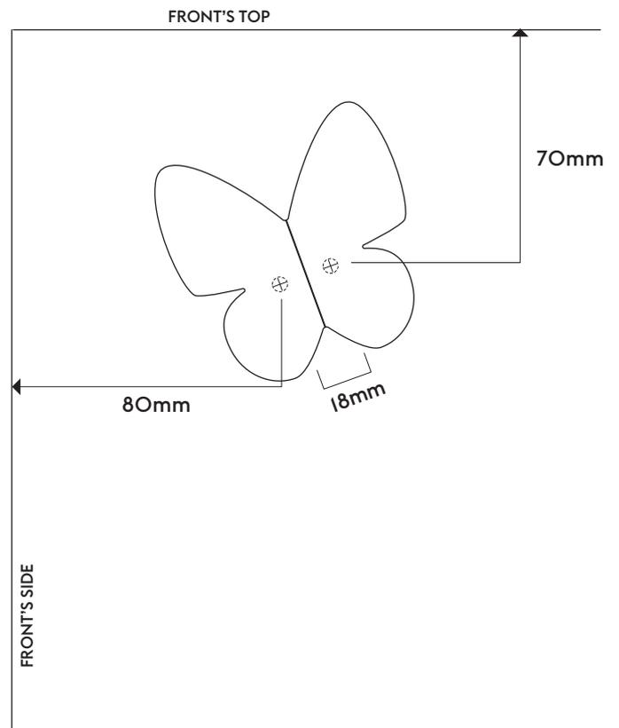
**TIP!** Drill the hole from the outside of the front. Hold a piece of wood tightly against the back of the front, for the drill to continue into. This will prevent the front from chipping on the back where the drill comes out.
