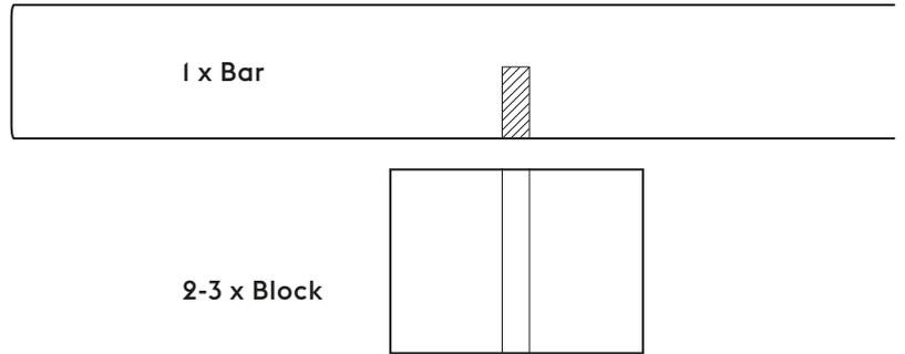
Bar 20 – Bar 80 = 2 blocks/screws/SuperWasher. Bar 80 – Bar 236 = 3 blocks/screws/SuperWasher.
